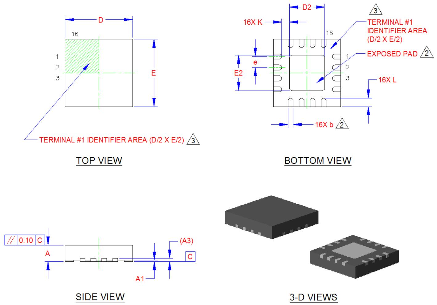
Figure 4 16-Pin QFN 4mm x 4mm Package Drawing
