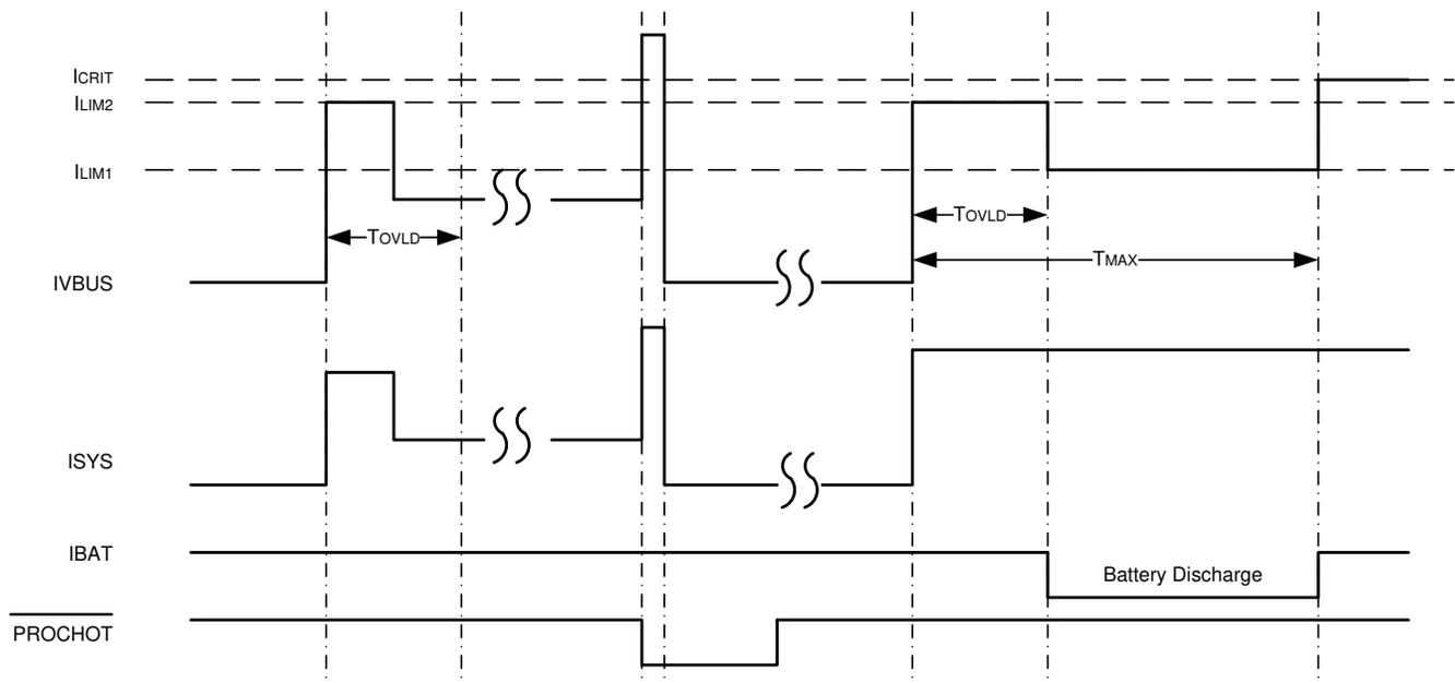
**Figure 9-1. Two-Level Adapter Current Limit Timing Diagram**
