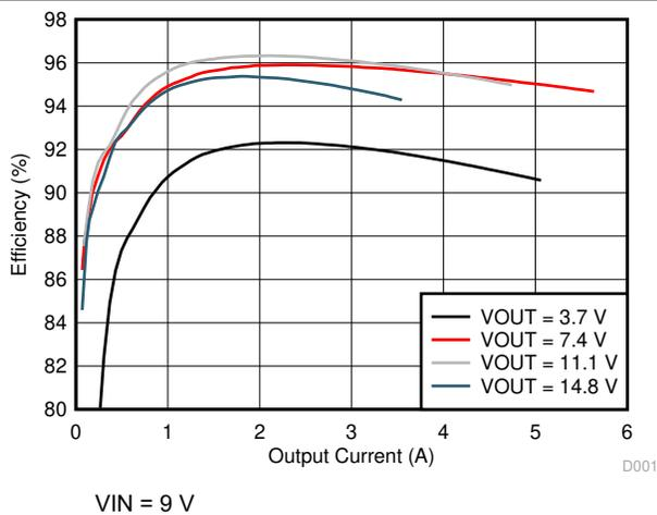
Figure 8-5. System Efficiency
