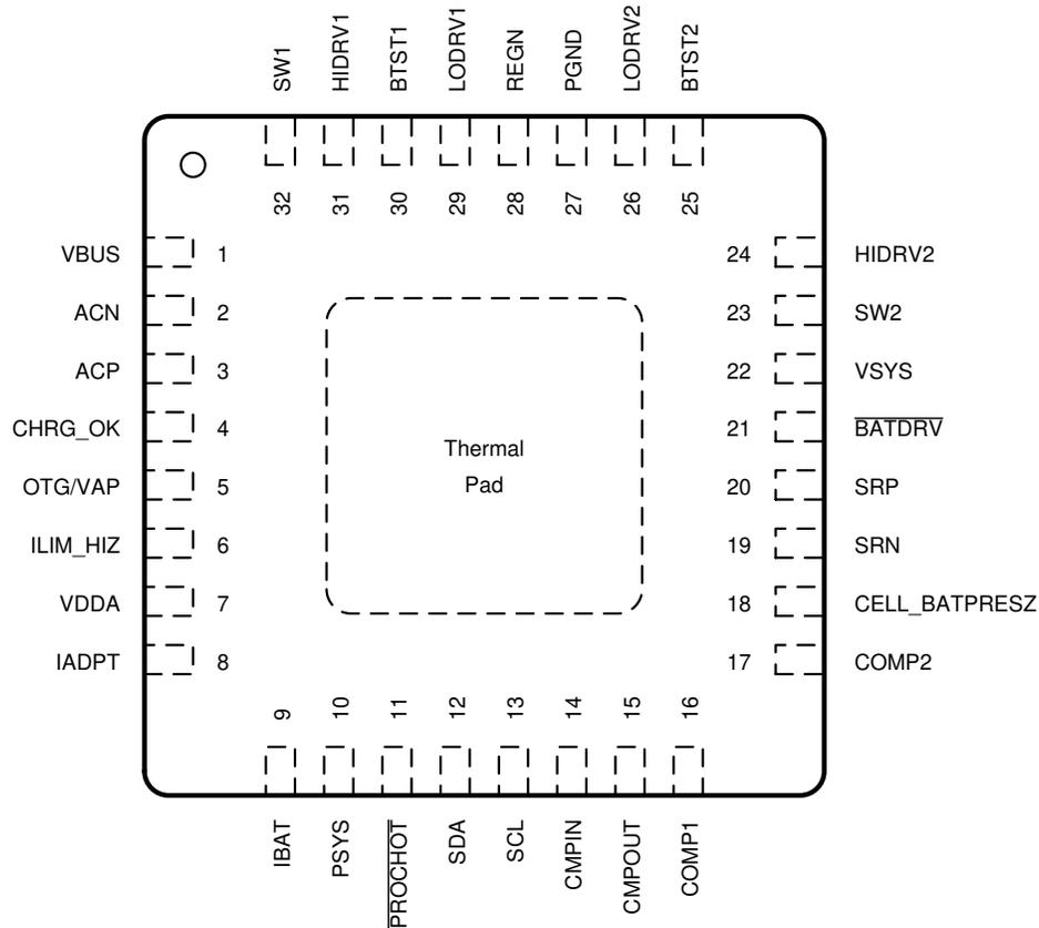
Figure 7-1. RSN Package 32-Pin WQFN Top View
