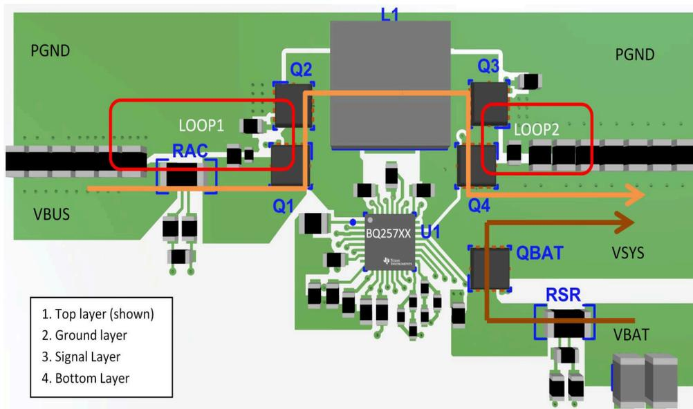
**Figure 12-1. Buck-Boost Charger Layout Reference Example Top View**
