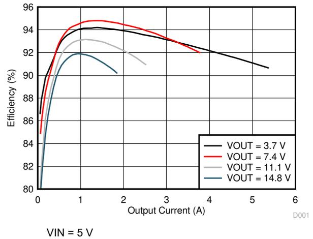
Figure 8-4. System Efficiency
