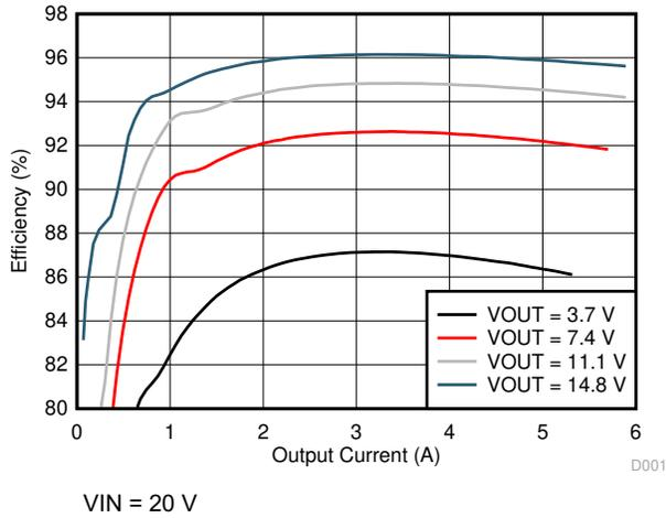
Figure 8-7. System Efficiency
