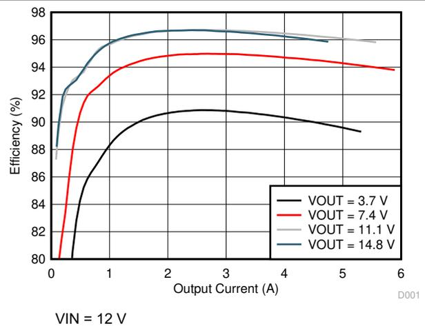
Figure 8-6. System Efficiency
