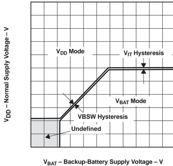
Figure 13. Normal Supply Voltage vs Backup-Battery Supply Voltage
