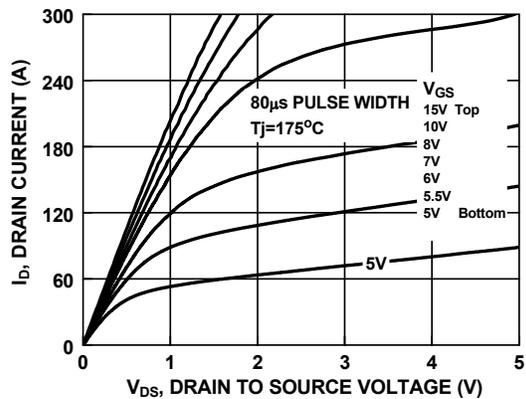
Figure 10. Saturation Characteristics
