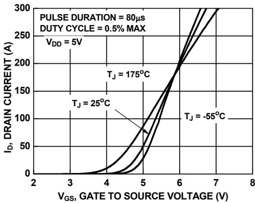
Figure 7. Transfer Characteristics
