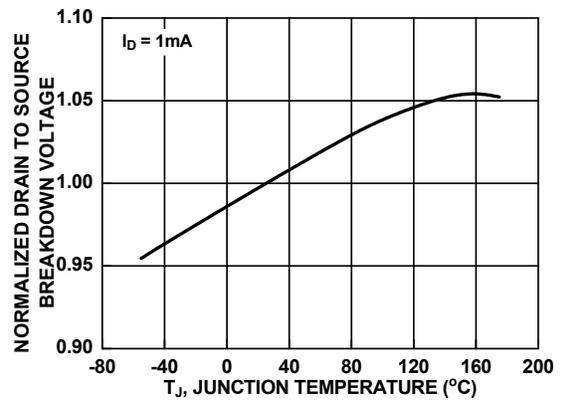
Figure 14. Normalized Drain-Source Breakdown Voltage vs. Junction Temperature
