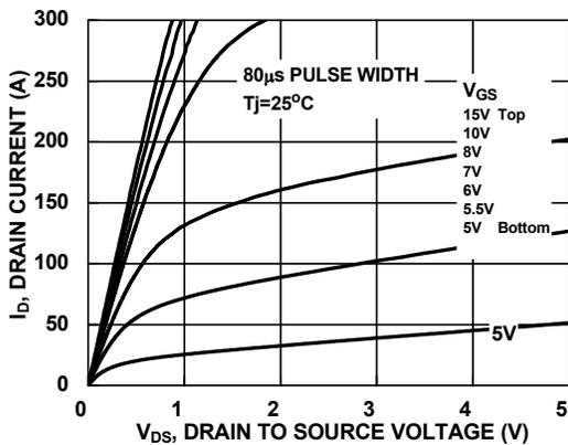
Figure 9. Saturation Characteristics
