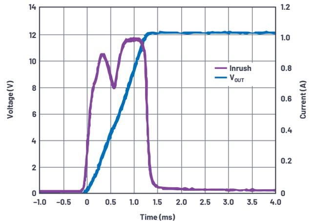
Figure 11. Inrush current limiting.
