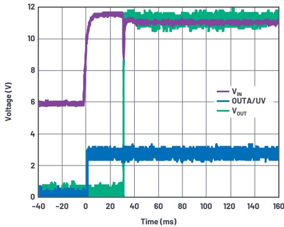
Figure 8. Expanded cranking recovery.
