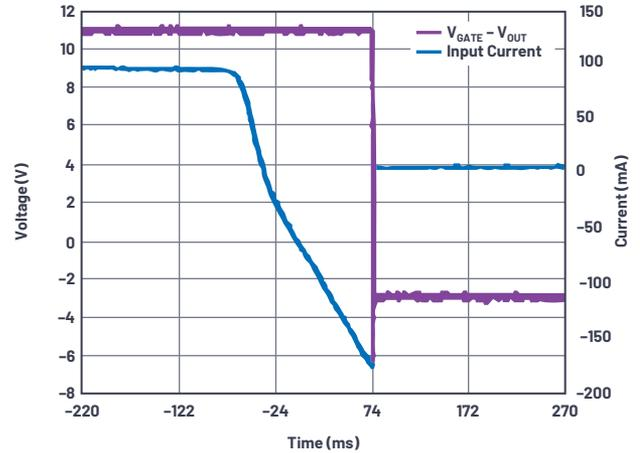
Figure 13. Assertion of reverse overcurrent protection.
