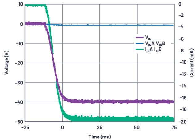
Figure 10. Reverse voltage protection measurement.
