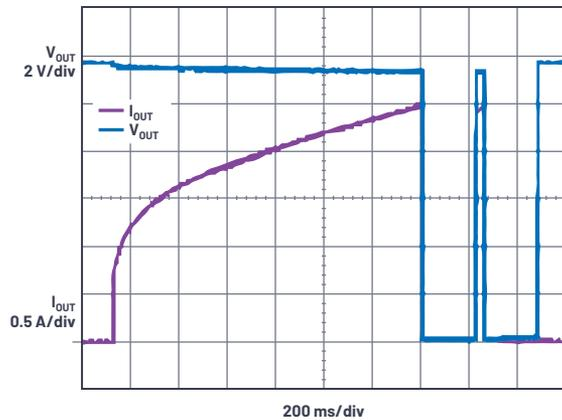
Figure 12. Assertion of forward overcurrent protection and retry delay.
