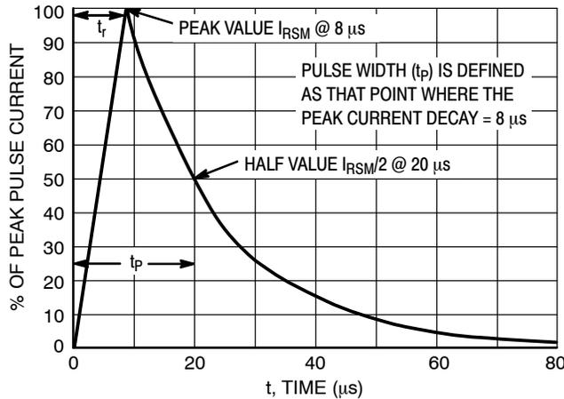
Figure 10. 8 x 20  $\mu s$  Pulse Waveform
