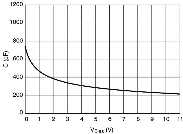
**Figure 5. CV Characteristics**
