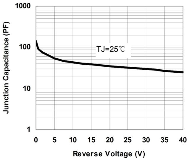
Fig.1-Typical Junction Capacitance
