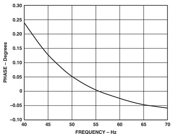
Figure 12. Phase Error between Channels (40 Hz to 70 Hz)
