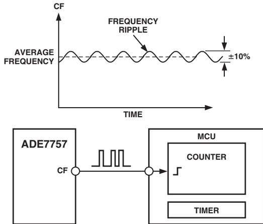
Figure 14. Interfacing the ADE7757 to an MCU
