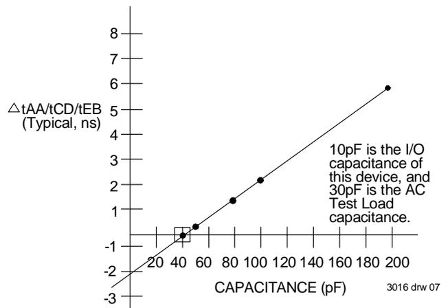
Figure 3. Lumped Capacitance Load Typical Derating Curve
