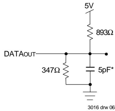
Figure 2. Output Test Load (for tCLZ, tBLZ, tOLZ, tCHZ, tBHZ, tOHZ, tWHZ, tCKHZ, and tCKLZ)
