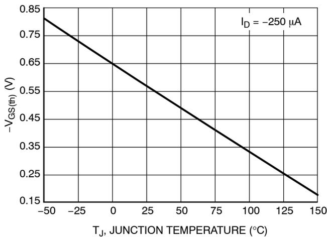
Figure 11. Threshold Voltage
