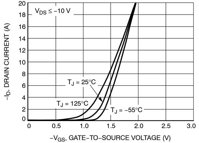
Figure 2. Transfer Characteristics
