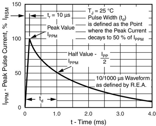
Fig. 3 - Pulse Waveform
