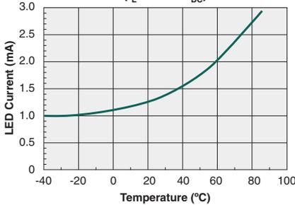
**Typical  $I_F$  for Switch Dropout vs. Temperature**
