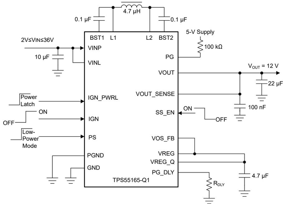
**Figure 9-4. TPS55165-Q1 Application Diagram for 12-V Voltage**
