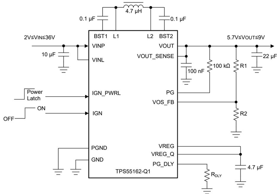
**Figure 9-2. TPS55162-Q1 Application Diagram for Adjustable Output Voltage**
