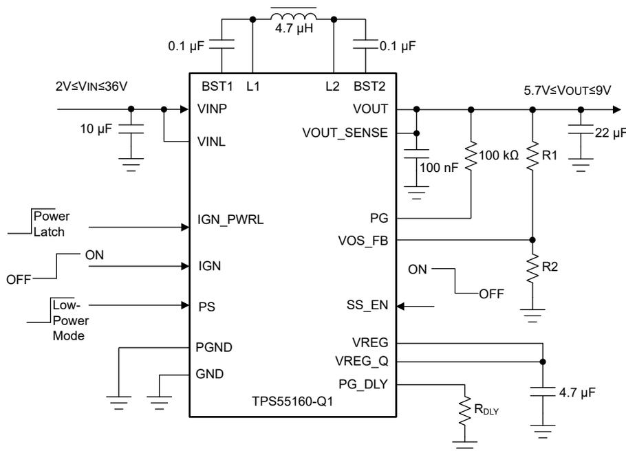
Figure 9-1. TPS55160-Q1 Application Diagram for Adjustable Output Voltage
