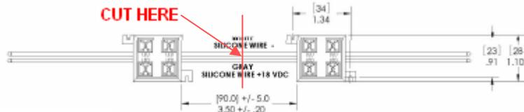
Modules can be secured onto a mounting surface with two #1 screws. Modules are waterproof and can be used outdoors. The installer is responsible for waterproofing the connection to the power source. The installer is also responsible for the use of an exterior approved power source.
