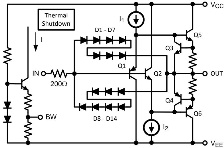
Figure 2. Simplified Circuit Diagram (Note: I<sub>1</sub> and I<sub>2</sub> are mirrored from I)
