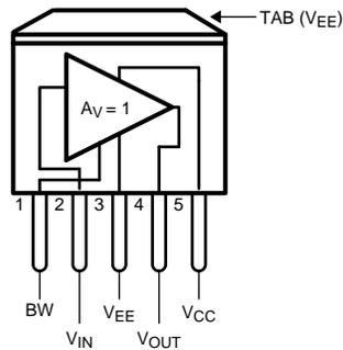
The KTT package is non-isolated package. The package's metal back and any heat sink to which it is mounted are connected to the same potential as the -V<sub>EE</sub> pin.
