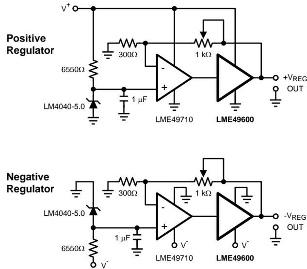
Figure 31. High Speed Positive and Negative Regulator
