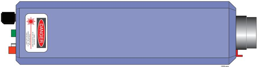
**Figure 7. Top view of laser showing the location of the “Warning logotype” label for a Class IIIa laser.**
