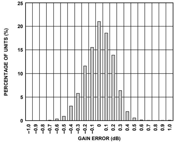
Figure 12. Gain Error Histogram,  $V_{\text{GAIN}} = 1.28$  V
