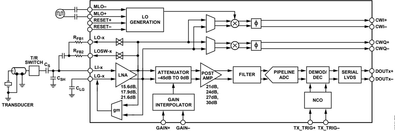
Figure 33. Simplified Block Diagram of a Single Channel
