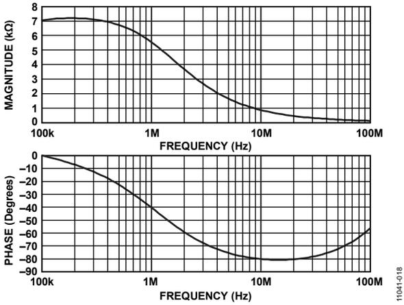
Figure 27. LNA Input Impedance Magnitude and Phase, Underterminated
