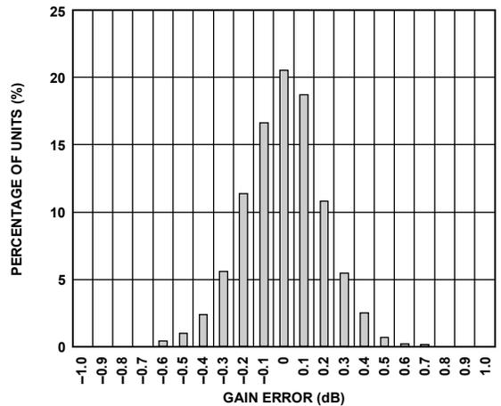
Figure 10. Gain Error Histogram,  $V_{\text{GAIN}} = -1.28$  V
