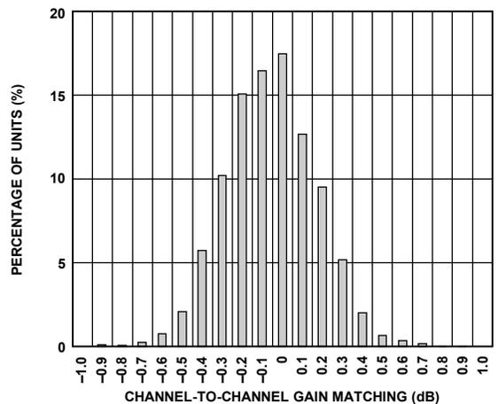
Figure 14. Gain Matching Histogram,  $V_{\text{GAIN}} = 1.2$  V
