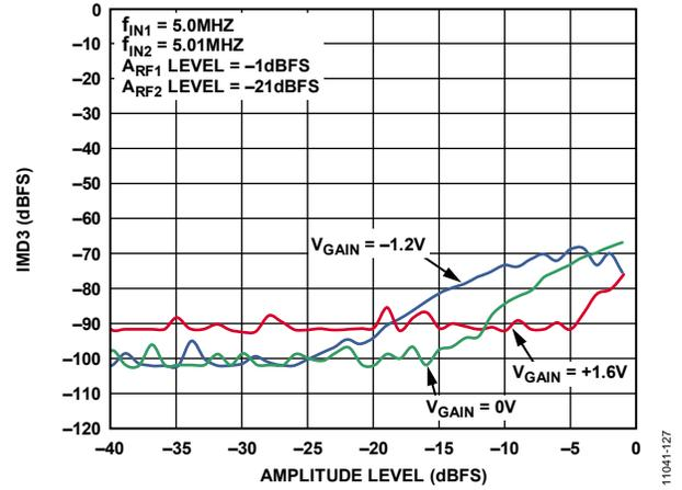
Figure 29. IMD3 vs. ADC Output Amplitude Level
