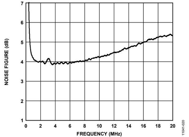
Figure 30. Noise Figure vs. Frequency, R<sub>S</sub> = R<sub>IN</sub> = 100Ω, LNA Gain = 17.9 dB, PGA Gain = 30 dB, V<sub>GAIN</sub> = 1.6 V
