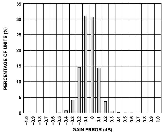
Figure 11. Gain Error Histogram,  $V_{\text{GAIN}} = 0$  V
