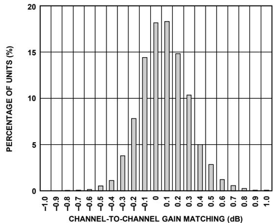
Figure 13. Gain Matching Histogram,  $V_{\text{GAIN}} = -1.2$  V
