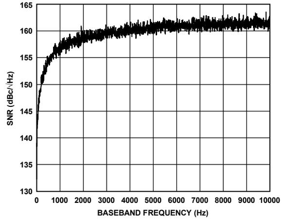
Figure 32. SNR vs. Baseband Frequency, -3 dBFS LNA Input
