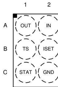
Top View = Xray through a soldered down part with A1 starting in upper left corner
