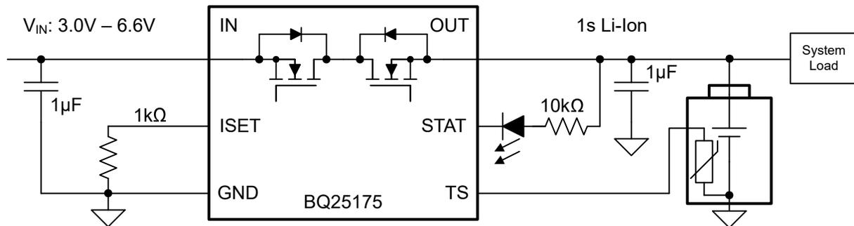
Figure 8-1. BQ25175 Typical Application for 1s Li-Ion Charging at 100 mA
