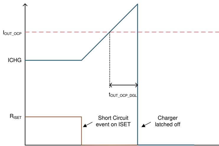
Figure 7-4. Overcurrent Protection
