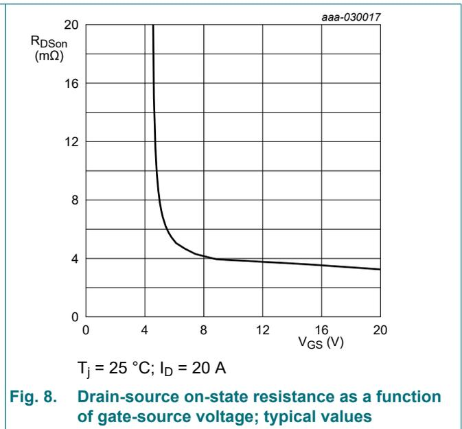
N-channel 40 V, 5 mΩ, standard level MOSFET in LPAK33 using NextPower-S3 technology
