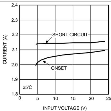
**Figure 29. Current Limit 1.8  $V_{OUT}$  at  $25^\circ\text{C}$**
