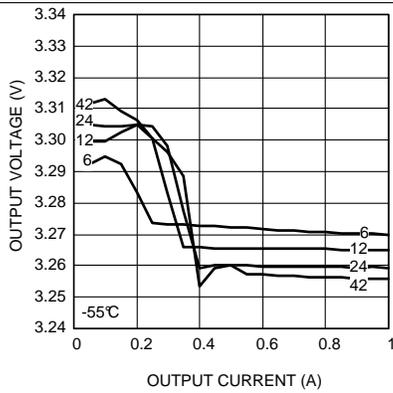
**Figure 25. Line and Load Regulation at  $-55^\circ\text{C}$**
