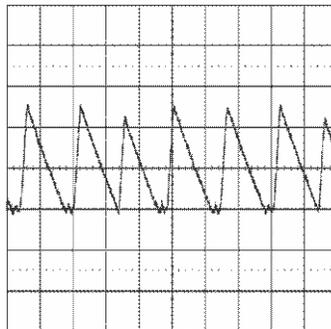
**Figure 36. Transition Mode Operation**
