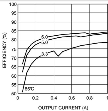
**Figure 21. Efficiency 42-V Input at 85°C**
