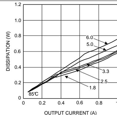
Figure 18. Dissipation 24-V Input at 85°C
