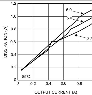
**Figure 22. Dissipation 42-V Input at 85°C**
