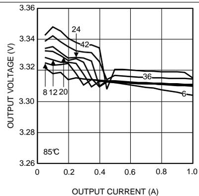
**Figure 24. Line and Load Regulation at 85°C**
