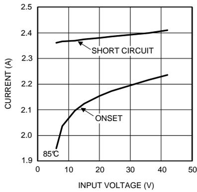
**Figure 31. Current Limit 3.3 V<sub>OUT</sub> at 85°C**
