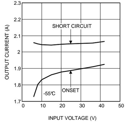
**Figure 32. Current Limit 3.3 V<sub>OUT</sub> at -55°C**
