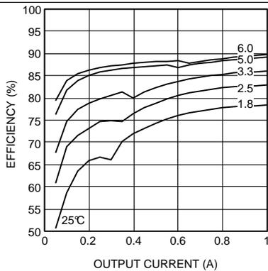
**Figure 5. Efficiency 24-V Input at 25°C**
