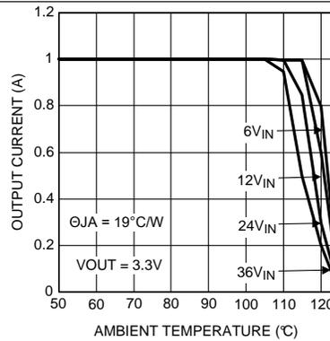
**Figure 28. Thermal Derating  $V_{OUT} = 3.3\text{ V}$**
