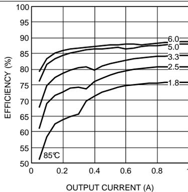
Figure 17. Efficiency 24-V Input at 85°C
