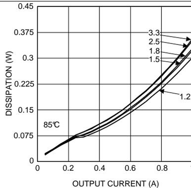
Figure 12. Dissipation 6-V Input at 85°C
