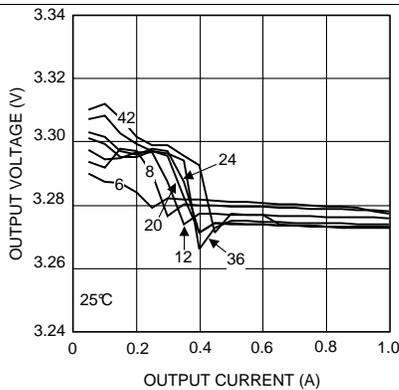
**Figure 23. Line and Load Regulation at 25°C**
