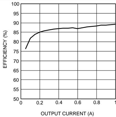
**Figure 37. Efficiency  $V_{IN} = 24\text{ V}$   $V_{OUT} = 5\text{ V}$**
