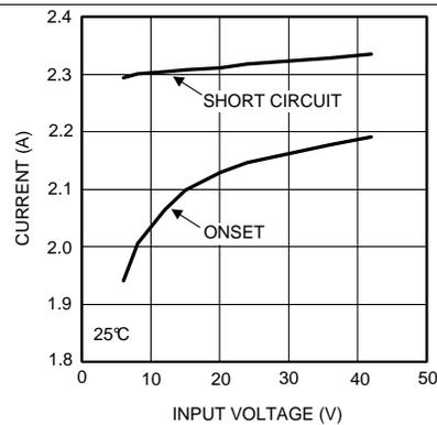
**Figure 30. Current Limit 3.3  $V_{OUT}$  at  $25^\circ\text{C}$**
