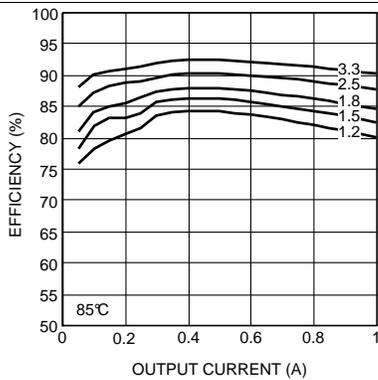
Figure 11. Efficiency 6-V Input at 85°C
