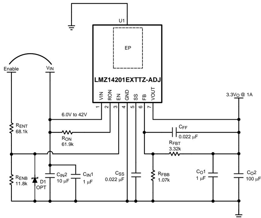
**Figure 34. Evaluation Board Schematic Diagram**
