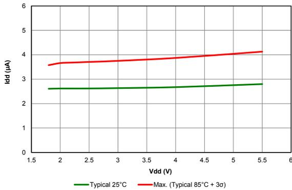
Figure 40-37. I<sub>DD</sub> TYPICAL, INT Oscillator
