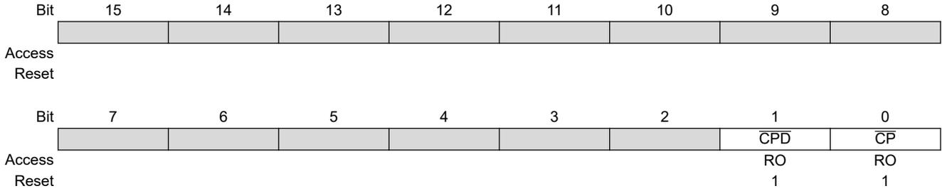
**Bit 1 –  $\overline{\text{CPD}}$**  Data NVM (DFM) Memory Code Protection bit
