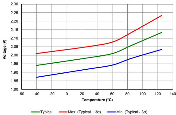
Figure 40-58. LOW POWER BROWN-OUT RESET REARM VOLTAGE
