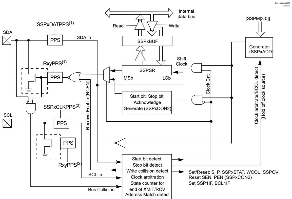
**Note 1:** SDA pin selections must be the same for input and output
