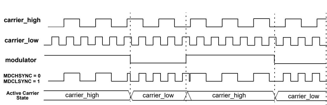
**Figure 26-6. Full Synchronization (MDCHSYNC = 1, MDCLSYNC = 1)**
