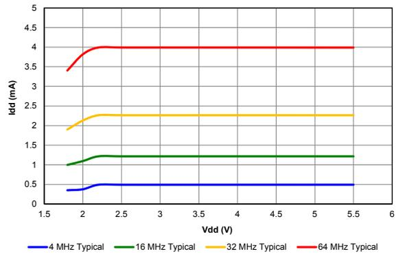
Figure 40-38. I<sub>DD</sub> MAXIMUM, INT Oscillator
