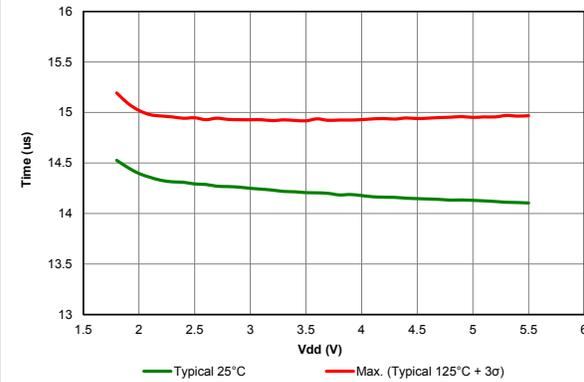
Figure 40-53. Wake From Sleep, VREGPM = 'b10, HFINTOSC = 4MHz
