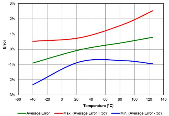
Figure 40-31. FVR Voltage Error 4x (Vdd = 5.5 V)
