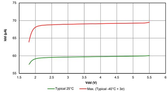
Figure 40-47. I<sub>PD</sub>, WATCH DOG TIMER (WDT)
