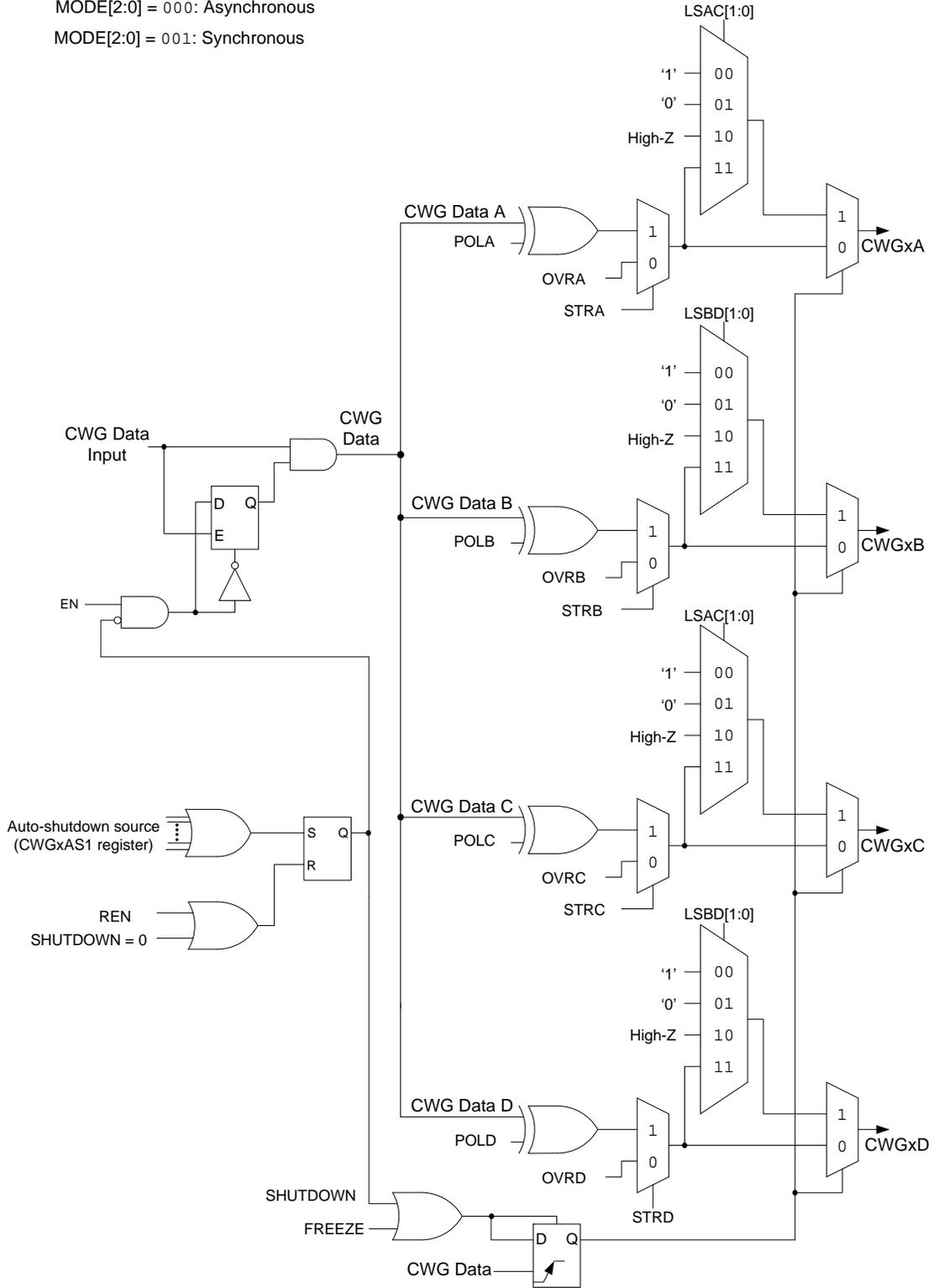
For example, when STRA = 0 then the corresponding pin is held at the level defined by OVRA. When STRA = 1, then the pin is driven by the modulated input signal.
