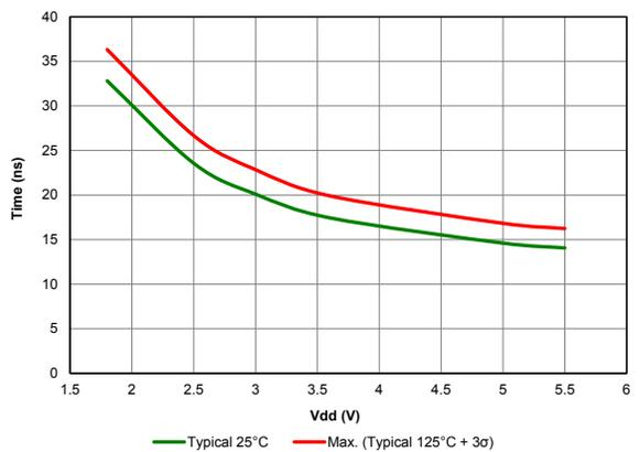
Figure 40-34. Rise time, slew rate control disabled
