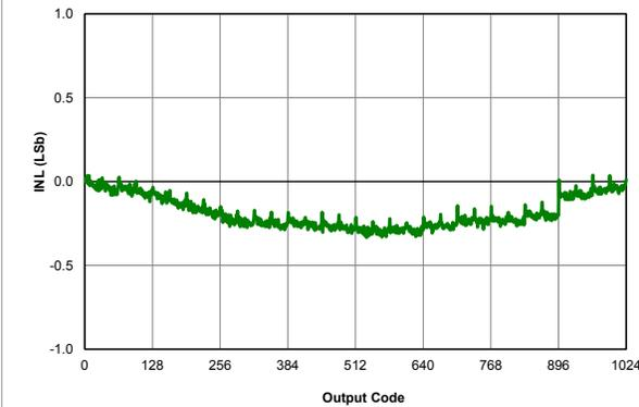
Figure 40-6. ADC, INL, Vdd = 3.0V, TAD = 4uS, 25C
