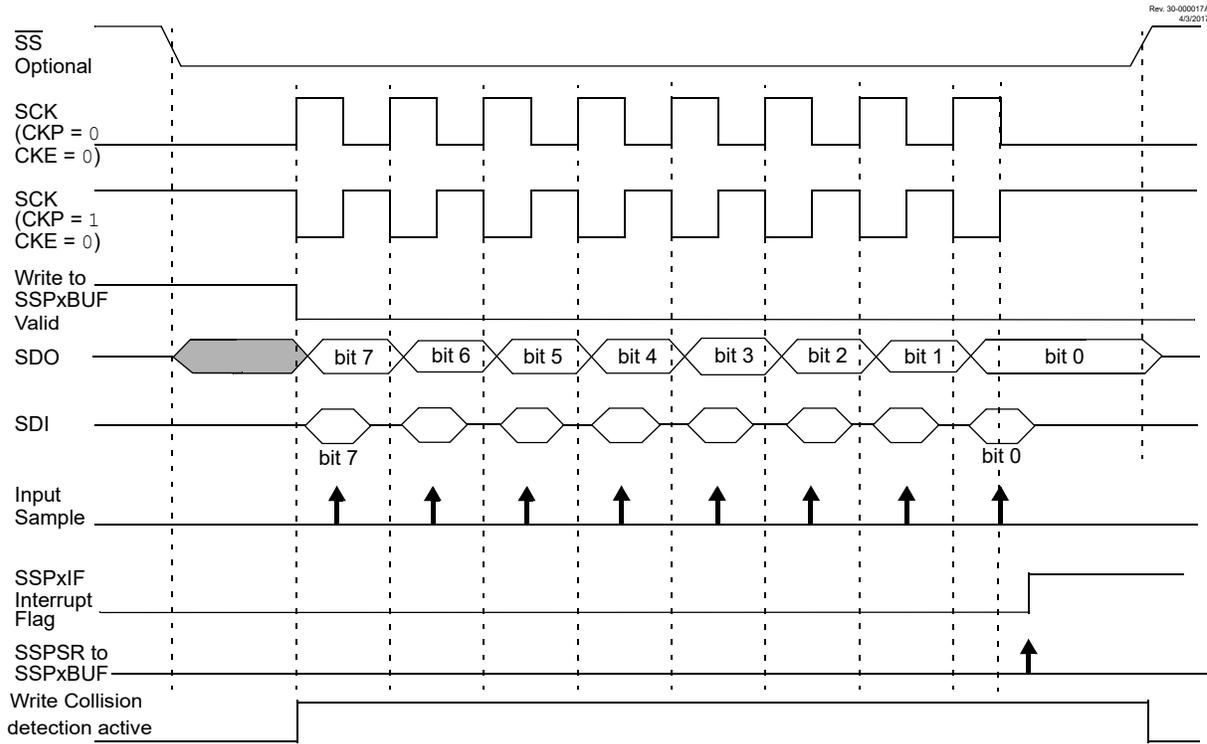
Figure 27-8. SPI Mode Waveform (Slave Mode with CKE = 1)
