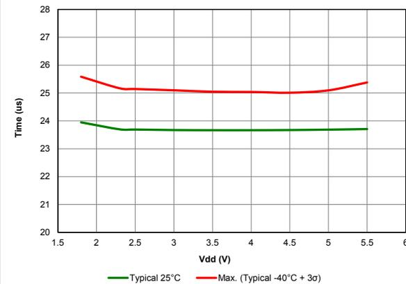
Figure 40-55. Wake From Sleep, VREGPM = 'b10, HFINTOSC = 16MHz
