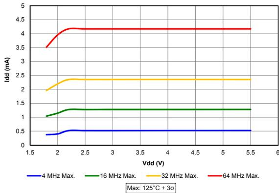
Figure 40-39. I<sub>DD</sub>, ECM OSCILLATOR, FOSC = 4 MHz
