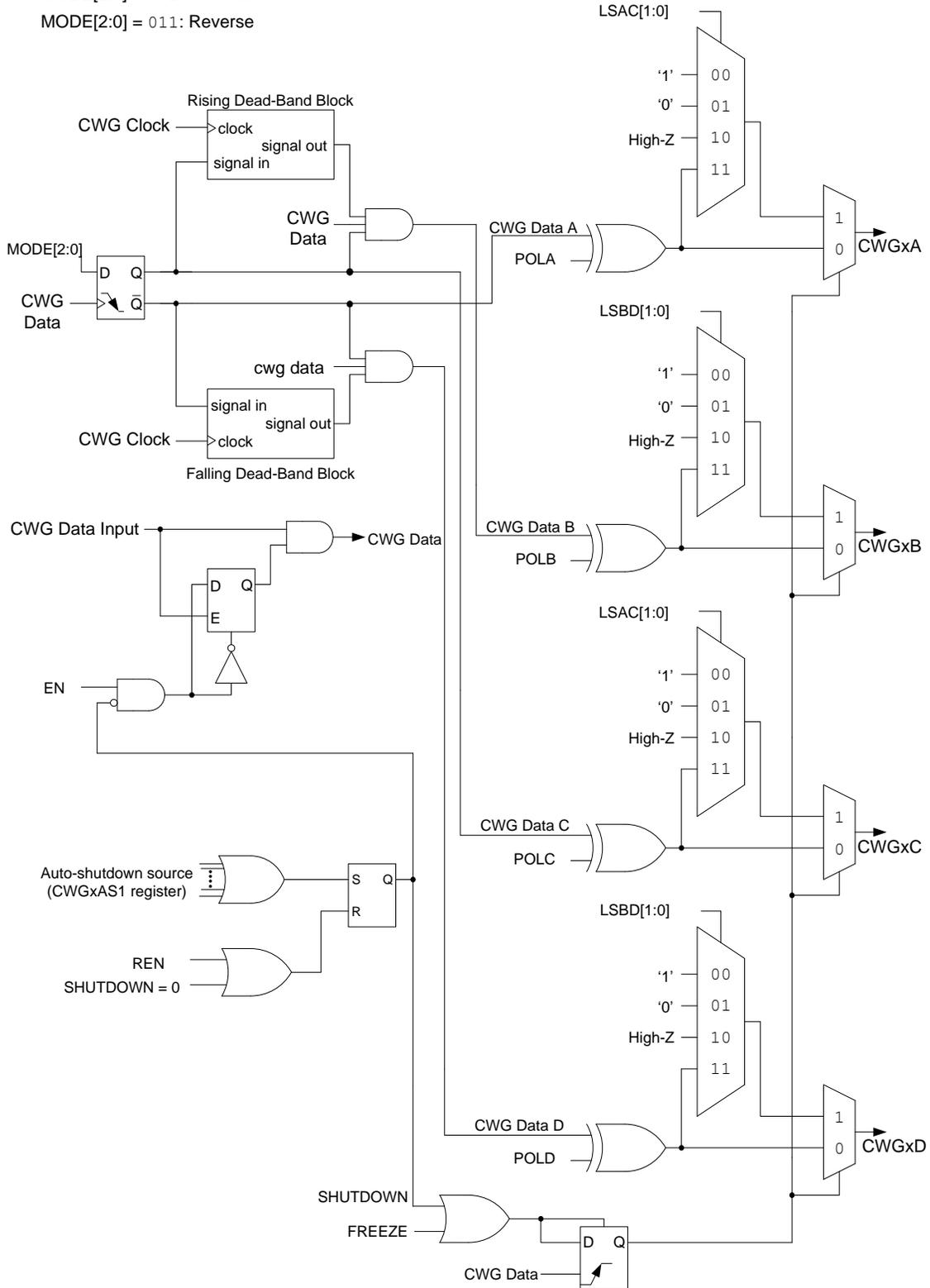
In Forward Full-Bridge mode (**MODE = 010**), CWGxA is driven to its Active state, CWGxB and CWGxC are driven to their Inactive state, and CWGxD is modulated by the input signal, as shown in Figure 24-7.
