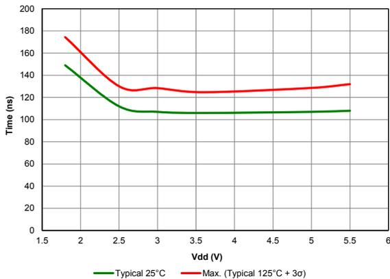
**Figure 40-28. Comparator Response Time Rising edge**
