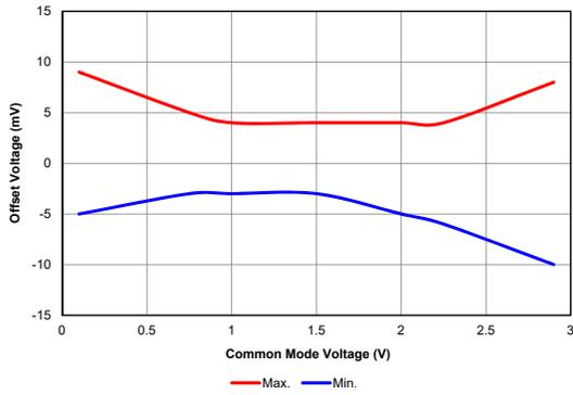
**Figure 40-24. COMPARATOR HYSTERESIS, NORMAL POWER MODE (CxSP = 1), Vdd = 5.5V, TYPICAL MEASURED VALUES**
