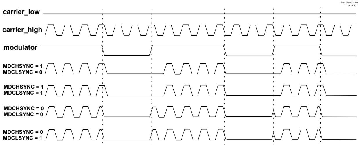
**Figure 26-3. No Synchronization (MDCHSYNC = 0, MDCLSYNC = 0)**
