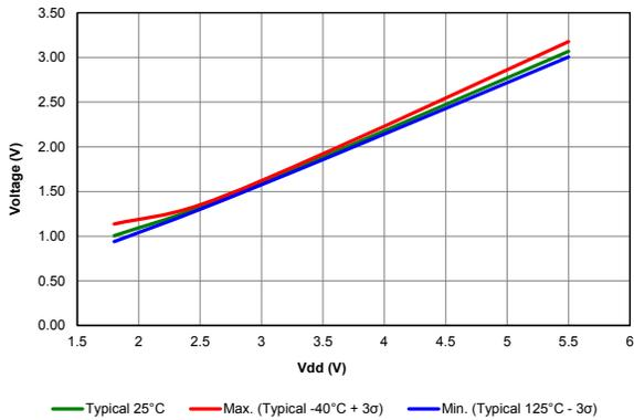
Figure 40-43. Schmitt Trigger Low Values
