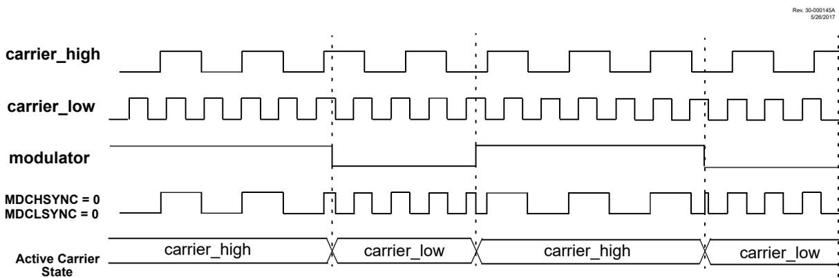
**Figure 26-4. Carrier High Synchronization (MDCHSYNC = 1, MDCLSYNC = 0)**
