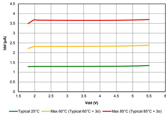
Figure 40-48. I<sub>PD</sub>, FIXED VOLTAGE REFERENCE (FVR)
