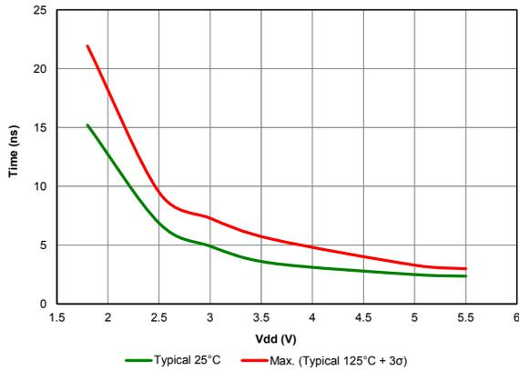
Figure 40-35. Fall time, slew rate control disabled
