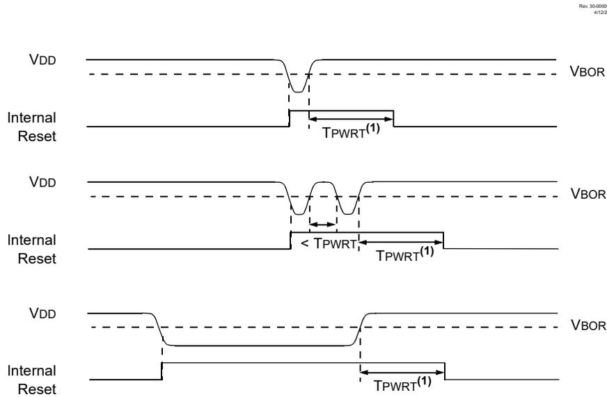
**Note:**  $T_{PWRT}$  delay only if  $\overline{PWRTE}$  bit is programmed to '0'.
