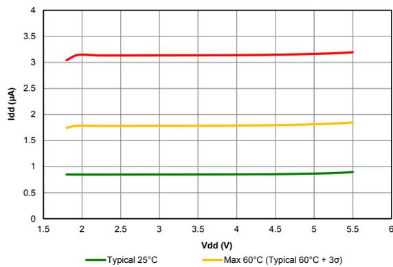
Figure 40-50. I<sub>PD</sub> BASE (VREGPM='b01)
