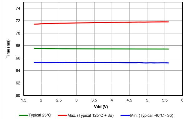
Figure 40-67. PWRT PERIOD vs. Temperature (V<sub>DD</sub> = 3.0V)
