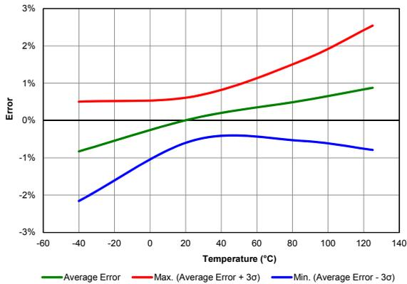
Figure 40-30. FVR Voltage Error 2x (Vdd = 5.5 V)
