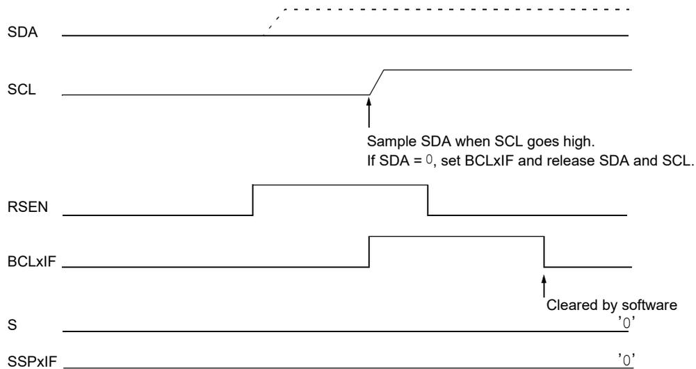
If SCL goes from high-to-low before the BRG times out and SDA has not already been asserted, a bus collision occurs. In this case, another master is attempting to transmit a data '1' during the Repeated Start condition, see Figure 27-37.
