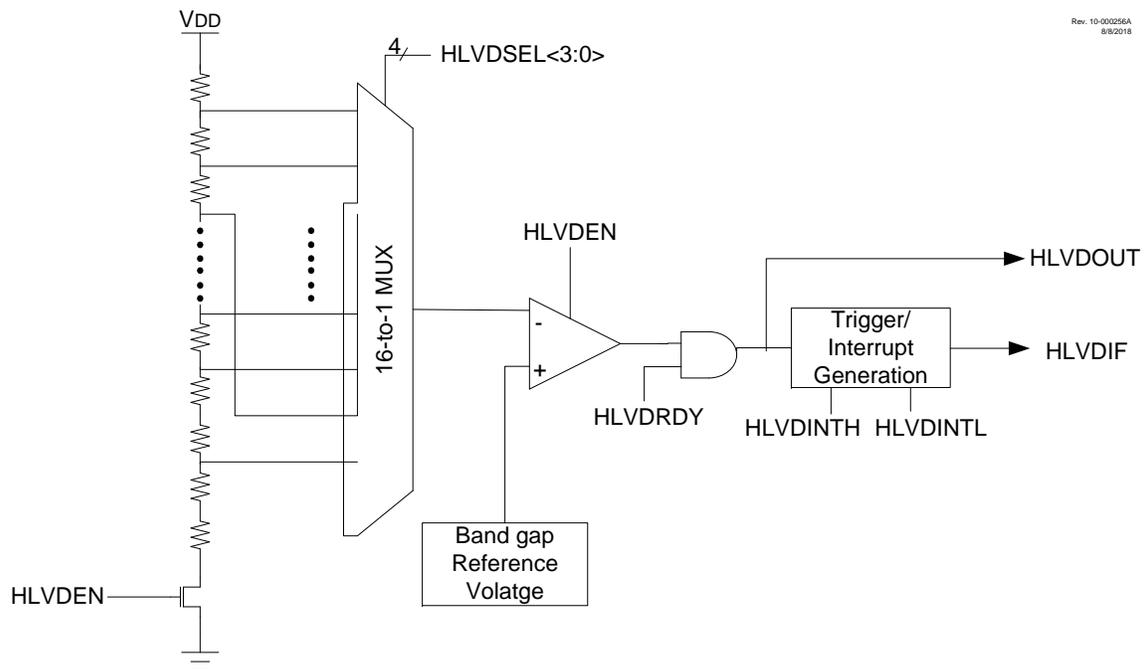
Since the HLVD can be software enabled through the HLVDEN bit, setting and clearing the enable bit does not produce a false HLVD event glitch. Each time the HLVD module is enabled, the **RDY** bit can be used to detect when the module is stable and ready to use.
