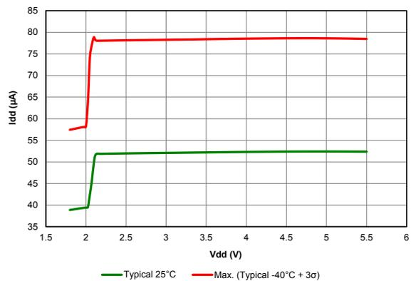
Figure 40-51. I<sub>PD</sub> BASE (VREGPM='b00)
