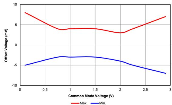
**Figure 40-23. COMPARATOR OFFSET, NORMAL POWER MODE (CxSP = 1), Vdd = 3.0V, TYPICAL MEASURED VALUES FROM -40°C to 125°C**
