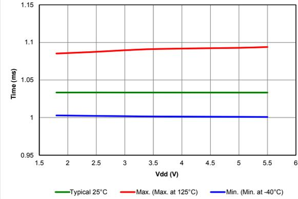
Figure 40-83. WDT BASE TIME-OUT PERIOD (WDTPS = 0, V<sub>DD</sub> = 3.0V)
