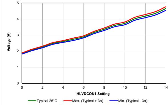
Figure 40-61. LVD Comparator Output Low Trip Points
