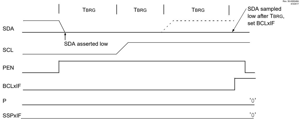
Figure 27-39. Bus Collision During a Stop Condition (Case 2)
