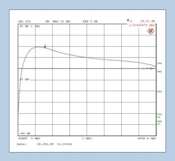
The picture left is the gain curve of BFP640F high linearity GPS LNA. LNA has 18.5dB gain, 0.9dB noise figure, and input third-order Intercept of +6dBm drawing 8mA from either 1.8 or 3.0V. 10 external components are used. Amplifier is unconditionally stable, e.g. k > 1,  $B_1 > 0$ . For more information please see application note AN121.
