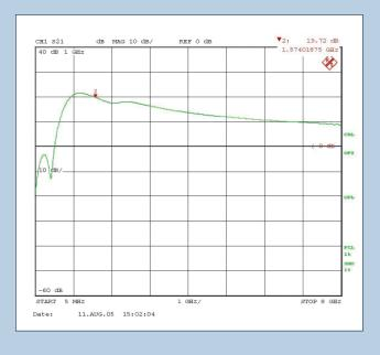
The picture left is the gain curve of BFP740F high Linearity GPS LNA. LNA has 20dB gain, 0.7dB noise figure, drawing 9mA from a 1.8 volt supply. 1.8 or 3.0V operation is possible with a single resistor value change. 10 external elements are used. Amplifier is unconditionally stable, e.g. k > 1,  $B_1 > 0$ . For more information please see application note AN117.
