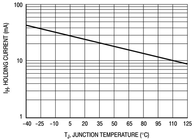
Figure 5. Typical Holding Current versus Junction Temperature
