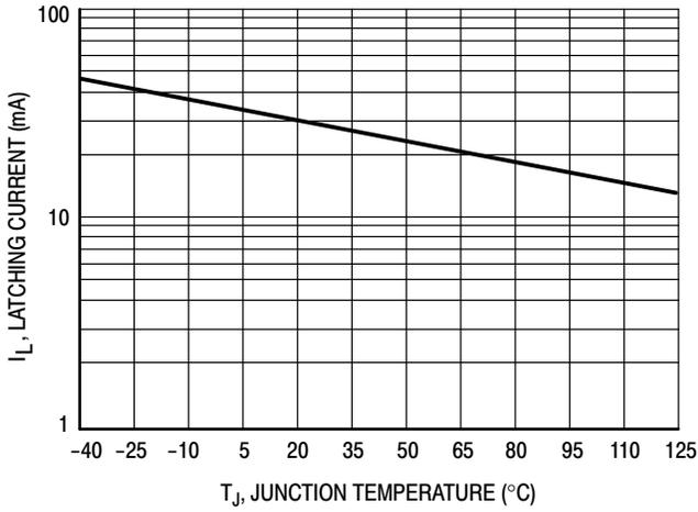
Figure 6. Typical Latching Current versus Junction Temperature
