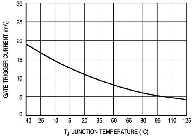
Figure 7. Typical Gate Trigger Current versus Junction Temperature
