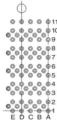
Recommended PCB hole mounting pattern for coaxial, column differential and stripline applications
