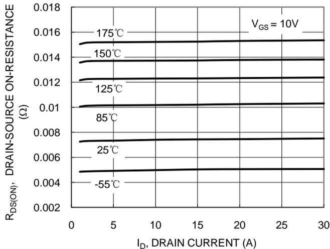
Figure 5. Typical On-Resistance vs. Drain Current and Temperature
