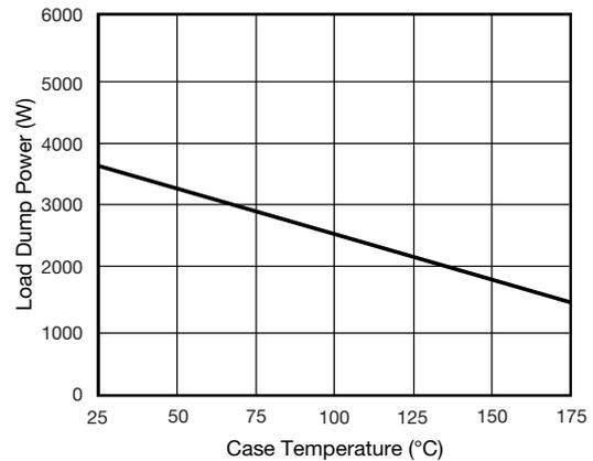
Fig. 2 - Load Dump Power Characteristics (10 ms Exponential Waveform)
