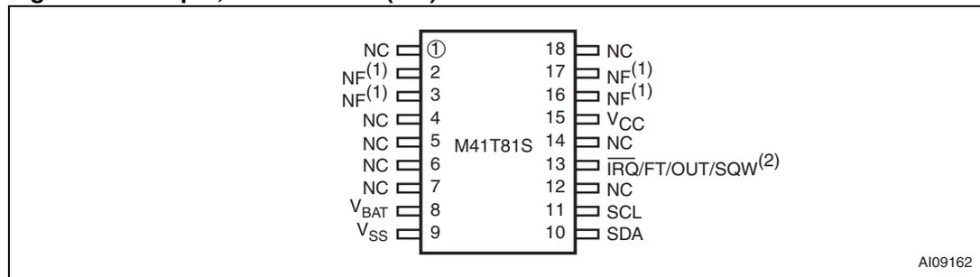
1. NC and NF pins should be tied to V<sub>SS</sub>. Pins 2 and 3 are internally shorted together. Pins 17 and 16 are internally shorted together.
