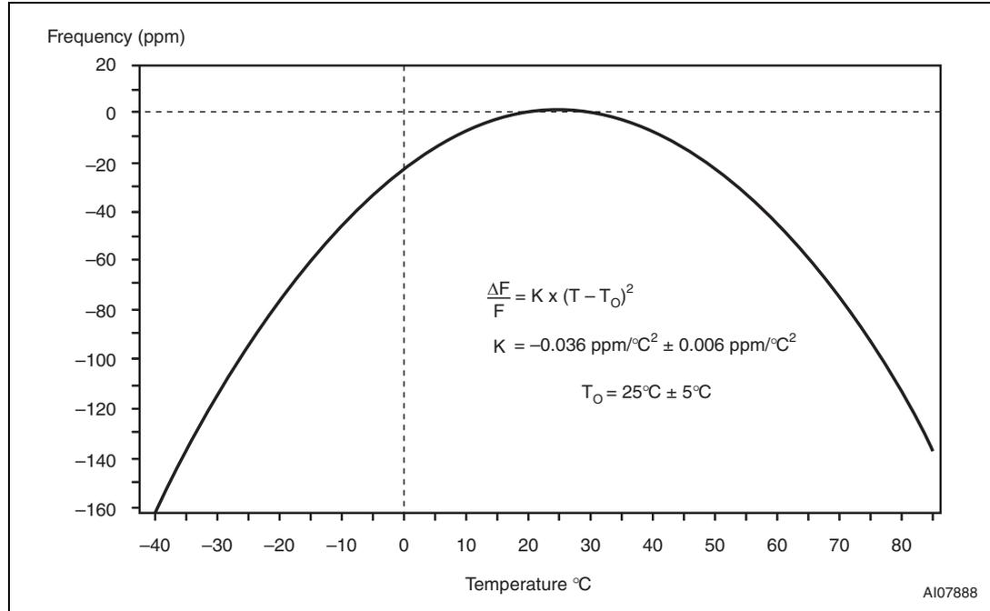
**Figure 12. Clock calibration**
